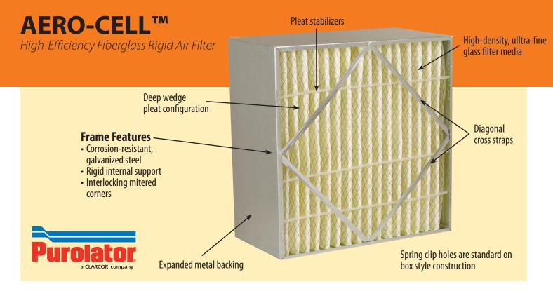
The AERO-CELL™ is a rigid air filter engineered to provide medium and high-efficiency filtration combined with a prolonged life cycle. Its box filter construction eliminates the need for retainers and special external wire media supports. A high surface area-to-depth ratio provides the maximum amount of effective filter media in areas of minimum in-line duct space. The result: A rigid, stable filter with consistent performance in a variety of operating conditions.
