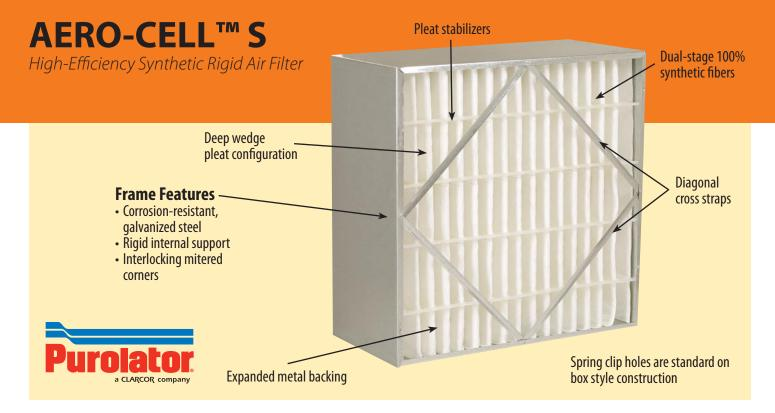
In an effort to respond to the increasing synthetic media requirements of the air filtration industry, Purolator offers the AERO-CELL S rigid box filter, a rigid air filter engineered to provide medium and high-efficiency filtration combined with a prolonged life cycle. Its box filter construction eliminates the need for retainers and special external wire media supports.
