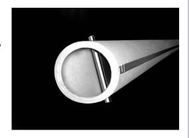
**Type T Core** (to fit Trane Company Roll Filter). Core is formed from 2-7/16" I.D. fiberboard tube. The tube contains a metal cup secured in each end recessed to a depth of 1-1/2" square.
