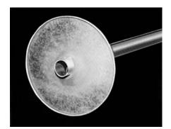
**Type B Core** (to fit BLC Industries Automatic Roll Machine). Core is constructed from 1-1/2" diameter: EMT conduit, with 11" diameter end plates recessed in approximately 1-3/8" from end of core.
