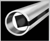
**Type CR Core** (to fit Carrier Corporation Series 31NA Roll Filter). Core is formed from a 2-7/16" fiberboard tube. The tube contains a metal cup secured in each end and recessed to a depth of 1-1/2". The cup is stamped to form a 1-1/2" square opening.
