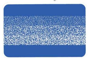
The Synthetic Media is constructed of high loft virgin polyester with gradient fiber density that permits even depth loading and long life.
