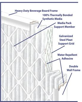
All DP filters are designed with a consistent pleat shape on predetermined centers causing dirt to collect evenly over the entire surface of the media. Fully utilizing every square inch of media results in a slow, steady rise in resistance for maximum dust holding capacity.
